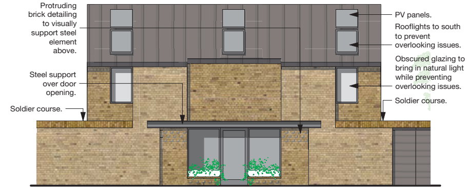
Scale: 1:100 Units Front/South Elevation
