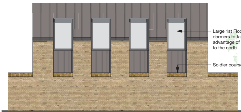
Scale: 1:100 Units Rear/North Elevation
